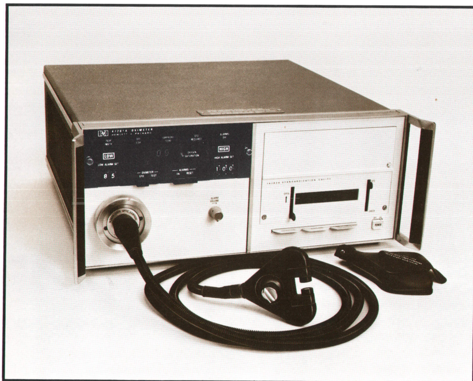
Fig. 1. Model 47201A Oximeter, shown here in the TEST mode with all alarm indicators illuminated, measures the percent saturation of hemoglobin continuously when the earprobe is properly placed on the ear. (The object shown to the right of the cable is the flexible light shield that covers the earprobe during a measurement.)
